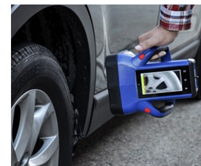
Portable X-ray backscatter imaging *Photograph courtesy of Viken detection.
