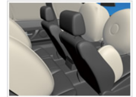
Air bags inflated using explosives technology
