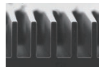
Enlarged image of developed Dry Film Resist
