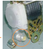
Micro gas generator
