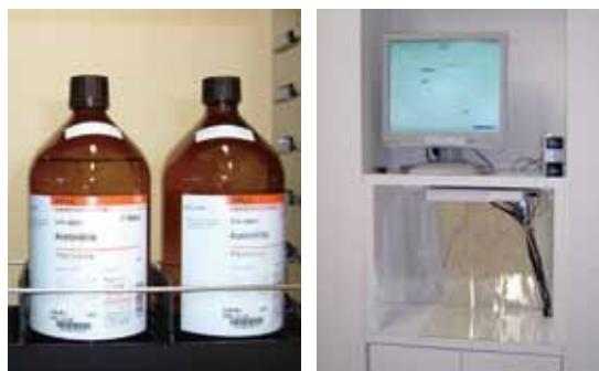
Storage container for hazardous substances with IC tag (left) and internal management system (right) (Integrated Research Building)
