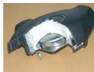
Inside of an air bag for driver's seats
